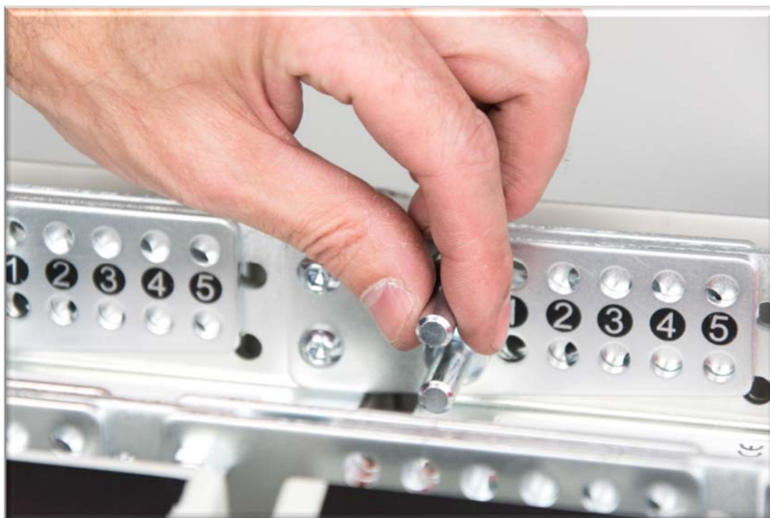
Adding the linking pins
