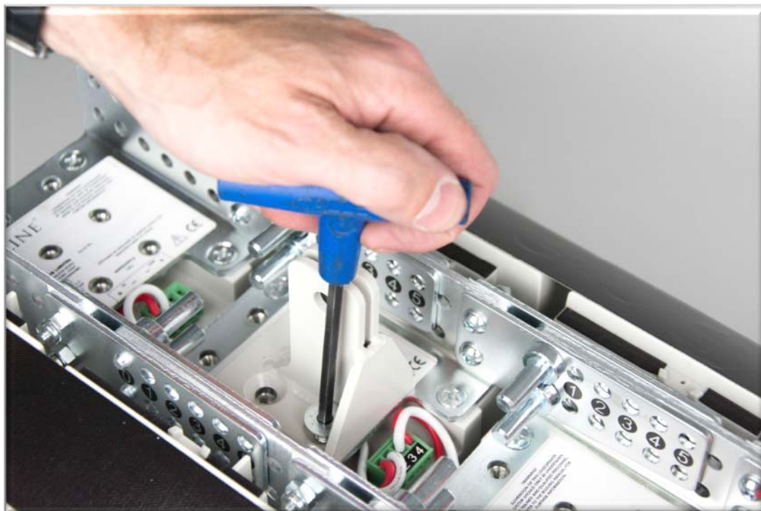
HAM03192 tie bracket in place
