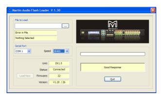
If the **Serial Speed** number is not set to 38400 to match the DX1.5 speed, the software lower right window may indicate **No Response**.
