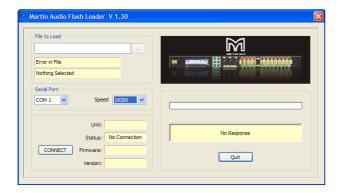
Make sure that the Serial port **Speed** on your pc screen is set to 38400 to match the DX1.5.
