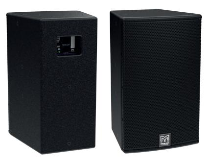
The PI10 is very compact, two-way passive loudspeaker designed for quality sound over short throw distances. It utilises a 10" (250mm)/2.5" (63mm) voice coil LF driver and a 1" (25mm) exit HF compression driver with a 1.4" (35mm) polyimide diaphragm.
