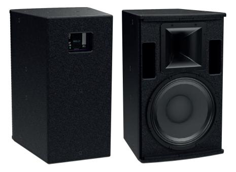
The PI12 is a high-performance, two-way system with a maximum SPL of 129dB peak @ 1m. It features a 12" (300mm)/2.5" (63mm) voice coil LF driver unit and a 1" (25mm) exit compression driver with a 1.4" (35mm) polyimide diaphragm on a rotatable  $80^{\circ}$  x  $50^{\circ}$  HF horn.
